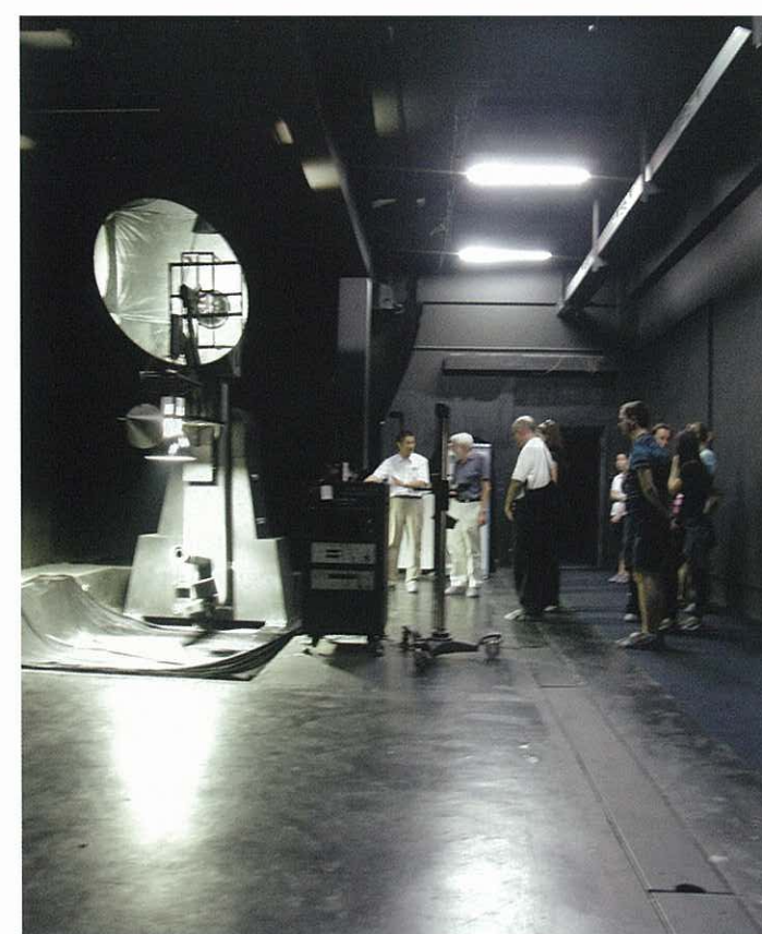
FIGURE 7. Boys’ toys: a goniophotometer at Everfine in Hangzhou. Photography is also difficult in black rooms!
