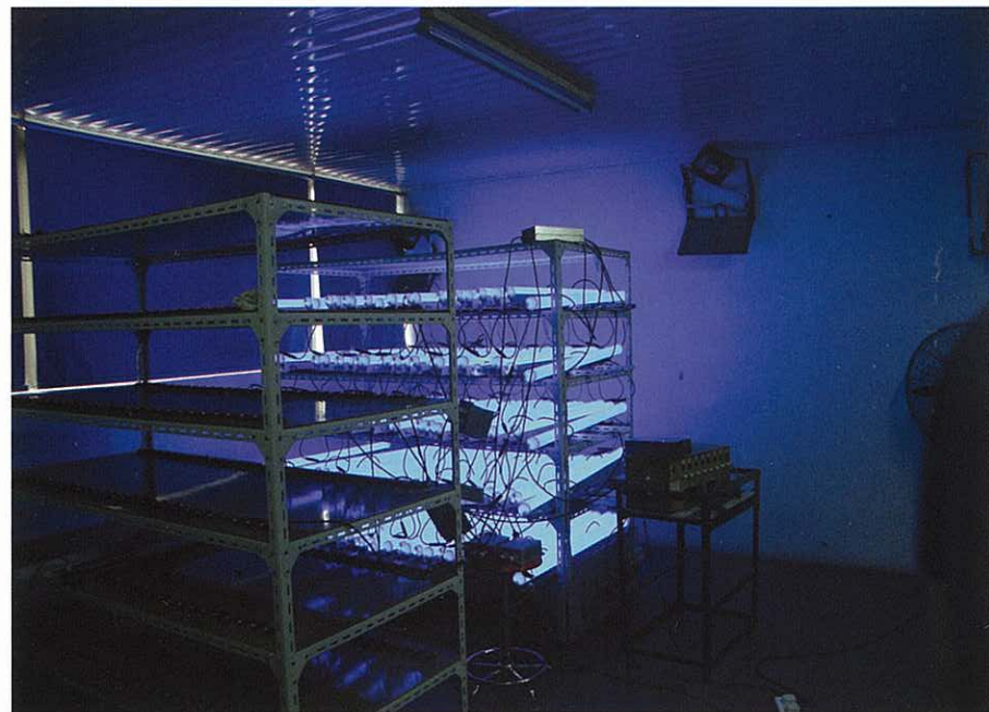
FIGURE 1. Soak testing blue LED outdoor tubes at RoLED creates an eerie atmosphere.
